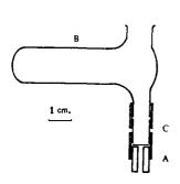
frequently results in disappointing losses of material owing to premature crystallisation during filtration or to repeated transferences of small quantities of solutions or solids from vessel to vessel. We have found that an apparatus, consisting essentially of a crystallisation vessel attached to a form of the Schwinger filter, is very convenient for repeated and rapid crystallisations. The principle of the apparatus is somewhat similar to that of the Bergkampf¹ filter-beaker.
